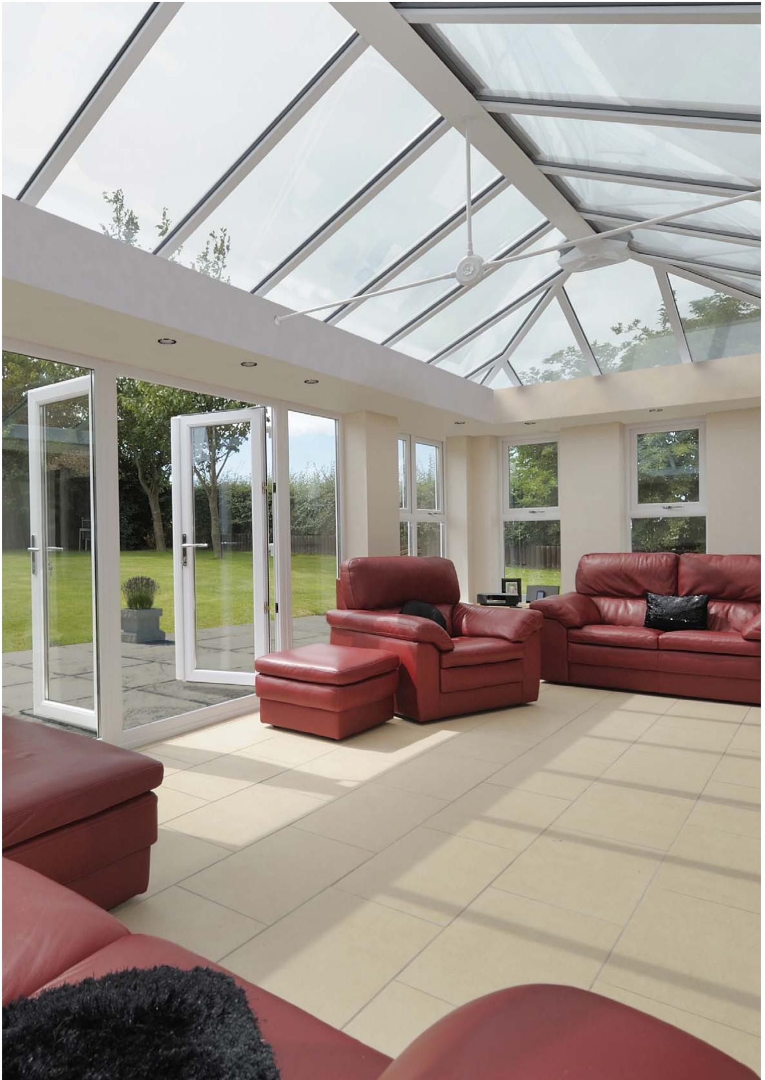
Livingroom uses an Ultraframe Classic glazed roof to which is attached a steel work ladder system at eaves and glazing bar positions. This is then plasterboarded and plaster skimmed to form a perimeter ceiling.
